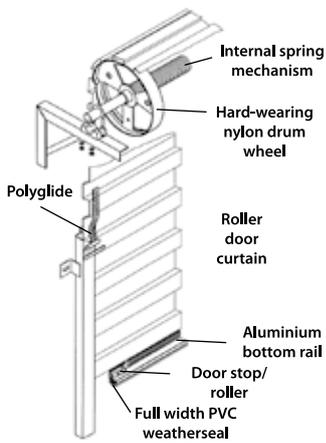
Gildermatic doors require an extra 20mm side clearance on the side the drive unit is required to be fitted.
